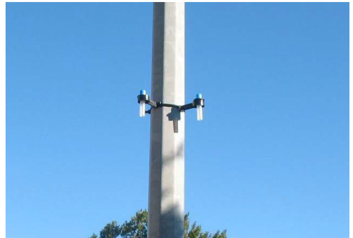
Figure 4: Photograph showing air quality diffusion tubes
